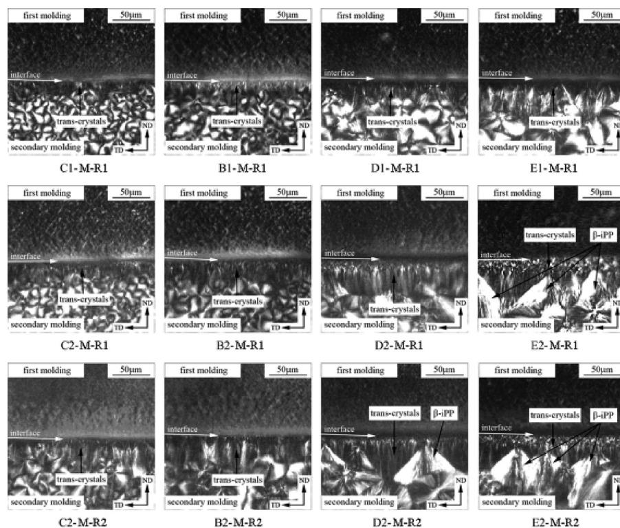
FIGURE 8. Optical micrographs near the interface obtained at different melt temperature and mold temperature at the same distance from the gate perpendicular to the flow direction (the secondary molding conditions B1, B2, C1, C2, D1, D2, E1, and E2, the cutting procedure M).
